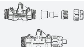
Install AC end cable on the other side of AC Trunk Cable (connected to the distribution box).
