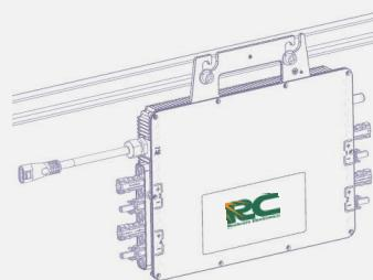
The AC cable contains earth wire, so grounding can be done directly with it.
