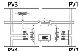
! Make sure the PVn+ and PVn- of the same PV channel is corresponding to the same PV panel or it will damage the inverter.
