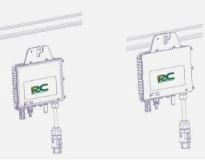
The AC cable contains earth wire, so grounding can be done directly with it.
