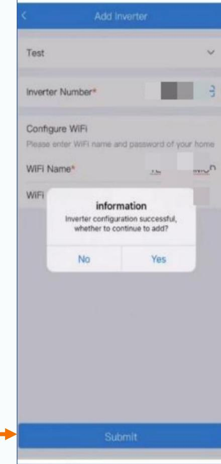
After creating the station, clicking magnifier button will search the inverters around the cell phone on-site. Then the app will list all available machines' serial numbers on-site(Grey serial number means it has been selected or registered in the other station). Check the serial number from machine's top side and select it from the app list. Please make sure number is correct.
