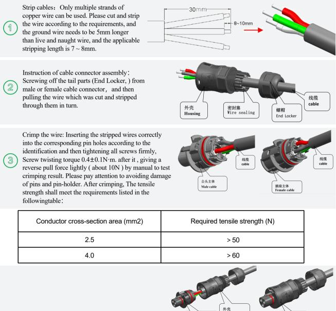
Install male & female cable body to plastic housing: Push the male or female cable body into housing body correctly according to the position of the clamping groove, and will hear a crisp "click" sound in place.
