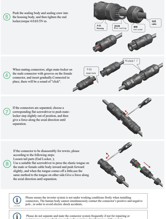
Please do not separate and mate the connector system frequently if not for repairing or maintenance reason which may reduce the waterproof performance of the system.
