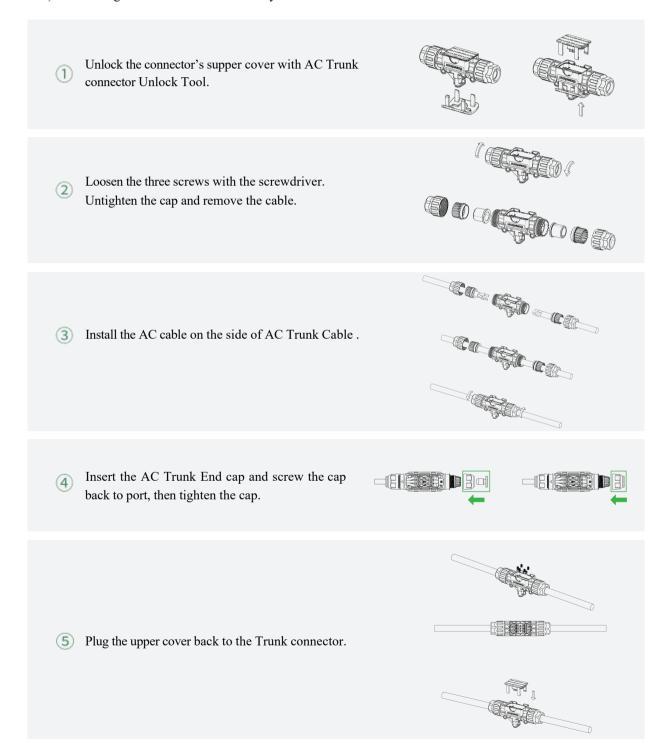
Install AC end cable on the other side of AC Trunk Cable (connected to the distribution box).
