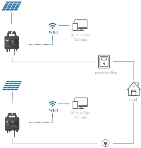
PV grid-connected system
